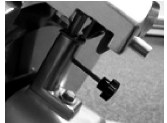
3. Secure the sharpening device to the machine by tightening the holder. Check to make sure that the sharpening device is well secured before using the machine.
